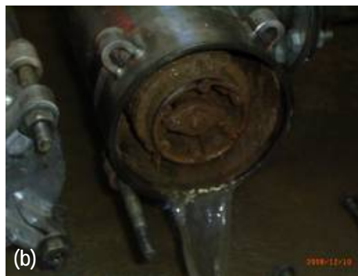
Fig 6: (a) Nyah pump station Victoria Australia (b) Membrane filter at Nyah from which Plumatella emarginata was first identified after the inaugural sampling tour conducted during the summer of December 2008
