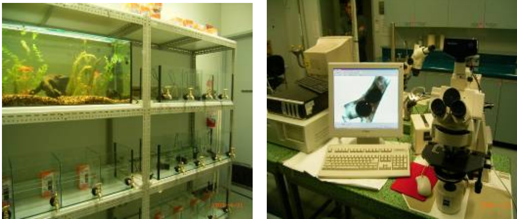
Fig 1: Bryozoan biofouling research station at the St Albans campus, Victoria University Australia. Note - the culture tanks have been compartmentalized into four sections to contain water from the four prime sampling sites – Ouyen, Kiamal, Piangil and Nyah in Victoria.
