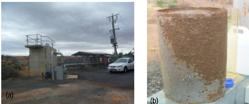
Fig 2: (a) Ouyen pump station Victoria, Australia (b) the clogged strainer at the Ouyen station from which Cordylophora caspia was first identified during the first summer sampling tour in December 2008.
