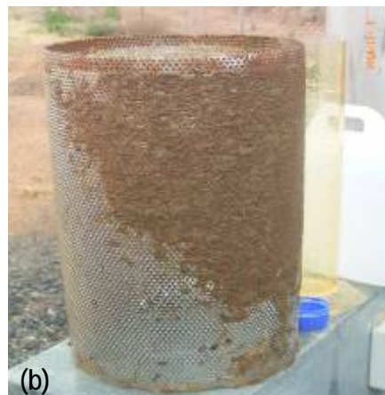
Fig 2: (a) Ouyen pump station Victoria, Australia (b) the clogged strainer at the Ouyen station from which Cordylophora caspia was first identified during the first summer sampling tour in December 2008.
