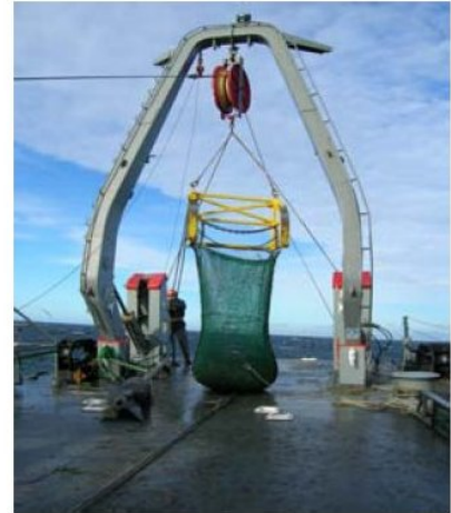
Figure 2. Agassiz dredge with a haul from 1000 m depth off the Concepción seep area, (Photo from COPAS Newsletter, March 2007).
